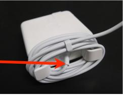
To reduce the strain on the cord, and prevent damage, it is recommended that you create some slack in the cord near the point where it connects to the charger brick. To do this, allow the first few inches at the base of the cord to stick out before you start to wrap the cord around the "wings".
