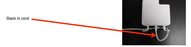
The picture below shows a cord wrapped up the recommended way.
